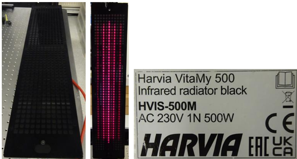
Figure 10: Harvia infrared heater VitaMy black glass HVIS-500M + grill (left), when operated (centre) and label (right). The radiator dimensions are 845 mm x 180 mm x 70 mm (height x width x depth).
