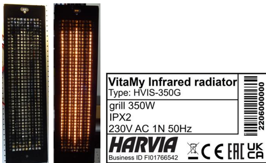
Figure 13: Harvia infrared heater VitaMy grill HVIS-350G (left), when operated (centre) and label (right). The radiator dimensions are 685 mm x 180 mm x 70 mm (height x width x depth).
