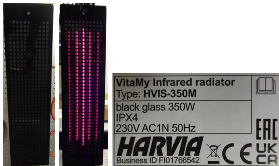
Figure 11: Harvia infrared heater VitaMy black glass HVIS-350M + grill (left), when operated (centre) and label (right). The radiator dimensions are 685 mm x 180 mm x 70 mm (height x width x depth).
