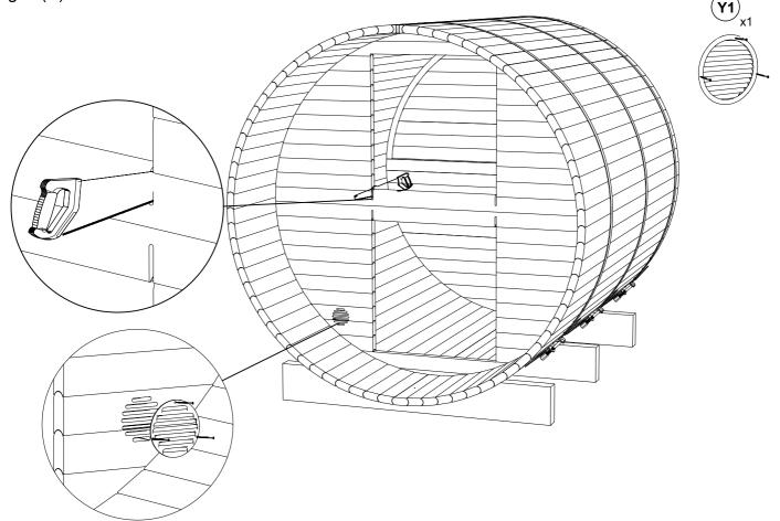
STEP 13: Pre-drill holes for screws. Fix both panels together using 5.0x120 (S4) screws.
