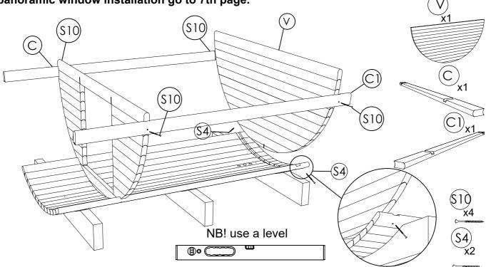
**STEP 6:** Continue placing body staves (C) tightly on both sides of the sauna using rubber mallet, and fixing body staves with screws 4.0x60(S10). Fix one stave higher on left side than at right.
