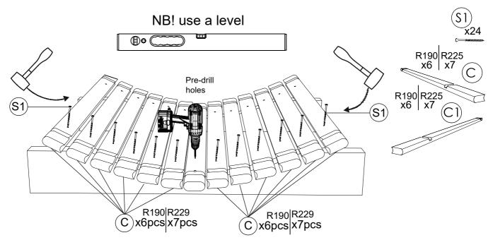
**STEP3:** Drill six 10 mm holes in front and back wall groove to the out-side in board connections as shown in the picture. Drill them in ≈30° angle. This will help drain excess water faster.
