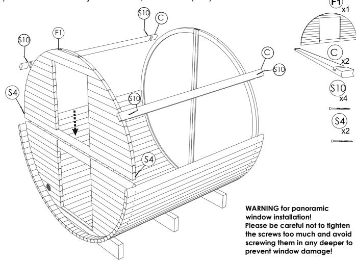
**STEP 7:** Place front top panel (F1) on front bottom panel (F), be sure panel is centered, leveled, completely seated. Fix panel using 5.0 x 120 (S4) screws on both sides.
