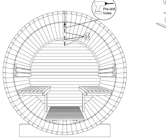
**STEP 22**: Install front and rear decorative roof finishing boards (W), fixing by screws 4.2x55(S7). Install porch benches (K), using screws 5.0 x 70 SS (S6) and 5.0 x 100 SS (S1). Hold the seat and leg assembly tight to the sauna wall. Using a level, make sure the bench seat is level from front to back. This will ensure proper placement.
