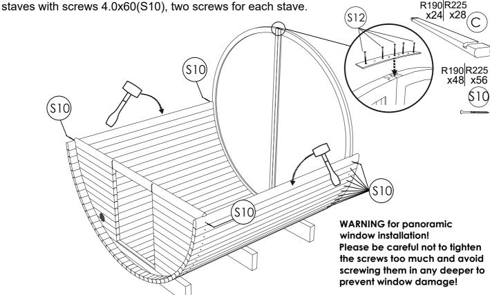
**STEP 8:** Take the upper front panel (F1) and place it on top of the front panel (F). Secure it by using 2 screws 5.0 x 120 (S4). Connect the panels (F1; V1) together by placing one body stave (C) on both sides where you can reach, with 4.0x60 (S10) screws.
