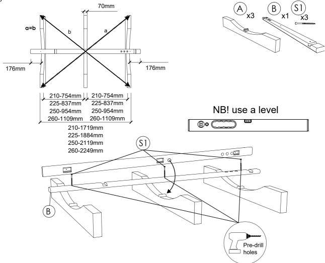
**STEP 2:** Pre-drill holes before fix staves with screws. Place 6 (R190) or 7 (R225) sauna body staves (C) to each side of the center stave (B)and fix with screws 5.0x100 SS (S1). Be sure to align the panel groove on every next body stave, to do that use rubber hammer.
