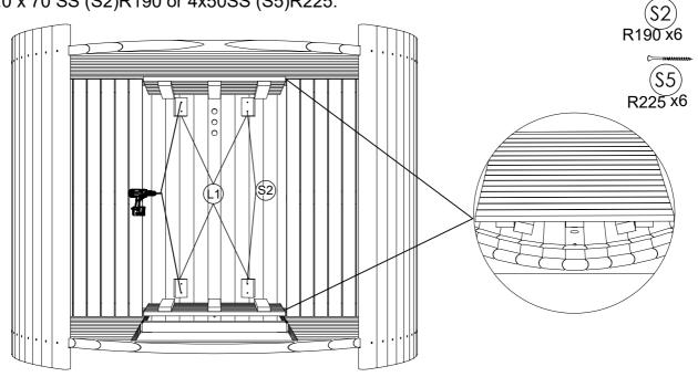
**STEP 20:** Pre-drill holes before fix with screws, install fixing blocks (L1) under floor duckboard using screw 4.0 x 70 SS (S2) R190 or 4x50SS (S5) R225. Place floor duckboards (L) on the floor and fix fixing blocks next to both flooring crossboards.
