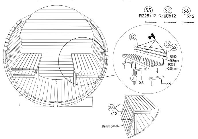
**STEP 19:** Place floor duckboards (L) to the both sides upwards and place fixing blocks next to the flooring cross boards. Pre-drill holes before fix with screws, install fixing blocks (L1) using screw 4.0 x 70 SS (S2)R190 or 4x50SS (S5)R225.
