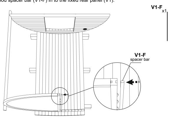
**STEP 6:**Apply silicone evenly in the groove of the second rear panel (V1). Place second rear panel (V1) in stave groove, be sure panel is centered, leveled, completely seated. Fix panel using 4.0 x 60 (S10) screw through last floor stave. Connect the panels (F; V1) together with body stave (C) with 4.0x60 (S10) screw.
