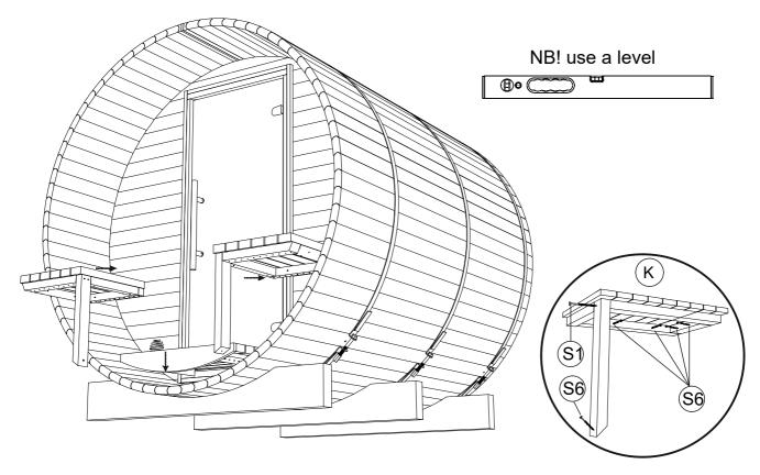
**STEP 23:** Pre-drill holes before fix stave with screws, install terrace roof trim (O1) in sauna with  $4.0 \times 50 \text{ SS } (S5)$  screws.
