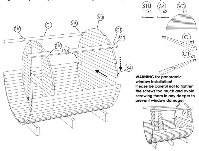
**STEP 9:** Continue placing body staves (C) tightly on both sides of the sauna using rubber mallet, and fixing body staves with screws 4.0x60(S10).
