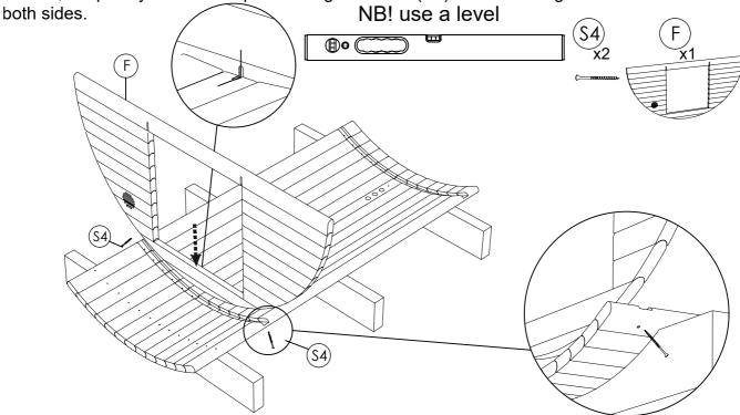
**STEP 5:** Place rear panel (V) in stave groove, be sure panel is centered, leveled, completely seated. Fix panel using 5.0 x 120 (S4) screws through last floor stave on both sides. **For full panoramic window installation go to 7th page.**
