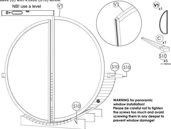
**STEP 7:** Fix Assembly tape with five 4x30 screws (S12) to fix both panels together. Continue placing body staves (C) tightly on both sides of the sauna using rubber mallet, and fixing body staves with screws 4.0x60(S10) two screws for each stave.
