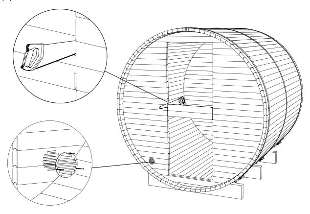
STEP 13: Pre-drill holes for screws. Fix both panels together using 5.0x120 (S4) screws.
