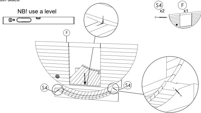
**STEP 5:** Place rear panel (V) in stave groove, be sure panel is centered, leveled, completely seated. Fix panel using 5.0 x 120 (S4) screws through last floor stave on both sides.
