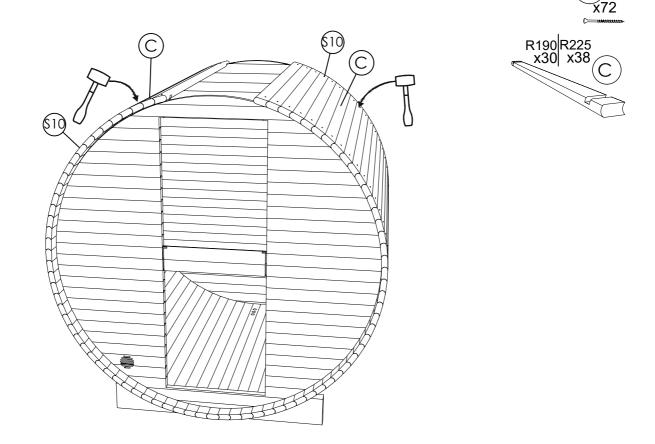
**STEP 10:** To finish the roof top joint, don't screw about last 2-3 boards (C) to each side, use roof finishing item (H). Different thickness filling pieces (H1) are provided to completely fill the gap. Once necessary parts are in, fix last boards with screws.
