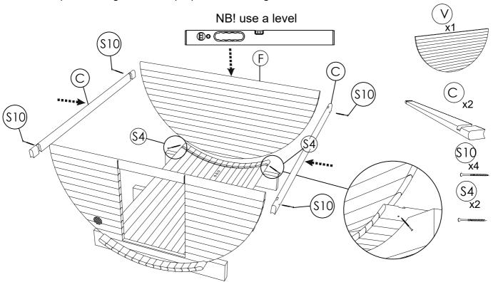
**STEP 6:** Continue placing body staves (C) tightly on both sides of the sauna using rubber mallet, and fixing body staves with screws 4.0x60(S10). Fix one stave higher on left side than at right.
