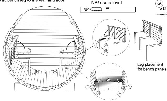
**STEP 18:** Pre-drill holes before fix backrest with screws, install backrests (J2) using screw  $4.0 \times 70 \text{ SS (S2)}$ . Fix sauna bench (J) to wall mounts and support leg using  $5 \times 70 \text{ SS (S6)}$  screws. Fix bench panel(if ordered) with screws  $4.0 \times 50 \text{ SS (S5)}$ .
