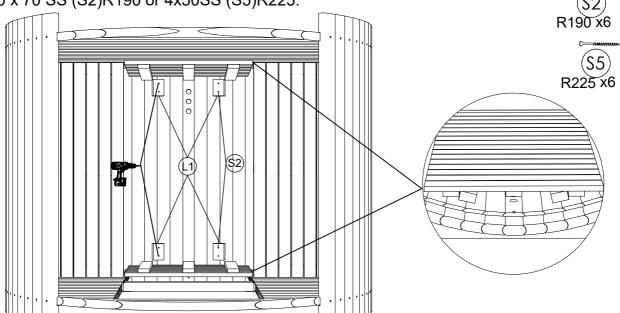
**STEP 20:** Pre-drill holes before fix with screws, install fixing blocks (L1) under floor duckboard using screw 4.0 x 70 SS (S2) R190 or 4x50SS (S5) R225. Place floor duckboards (L) on the floor and fix fixing blocks next to both flooring crossboards.
