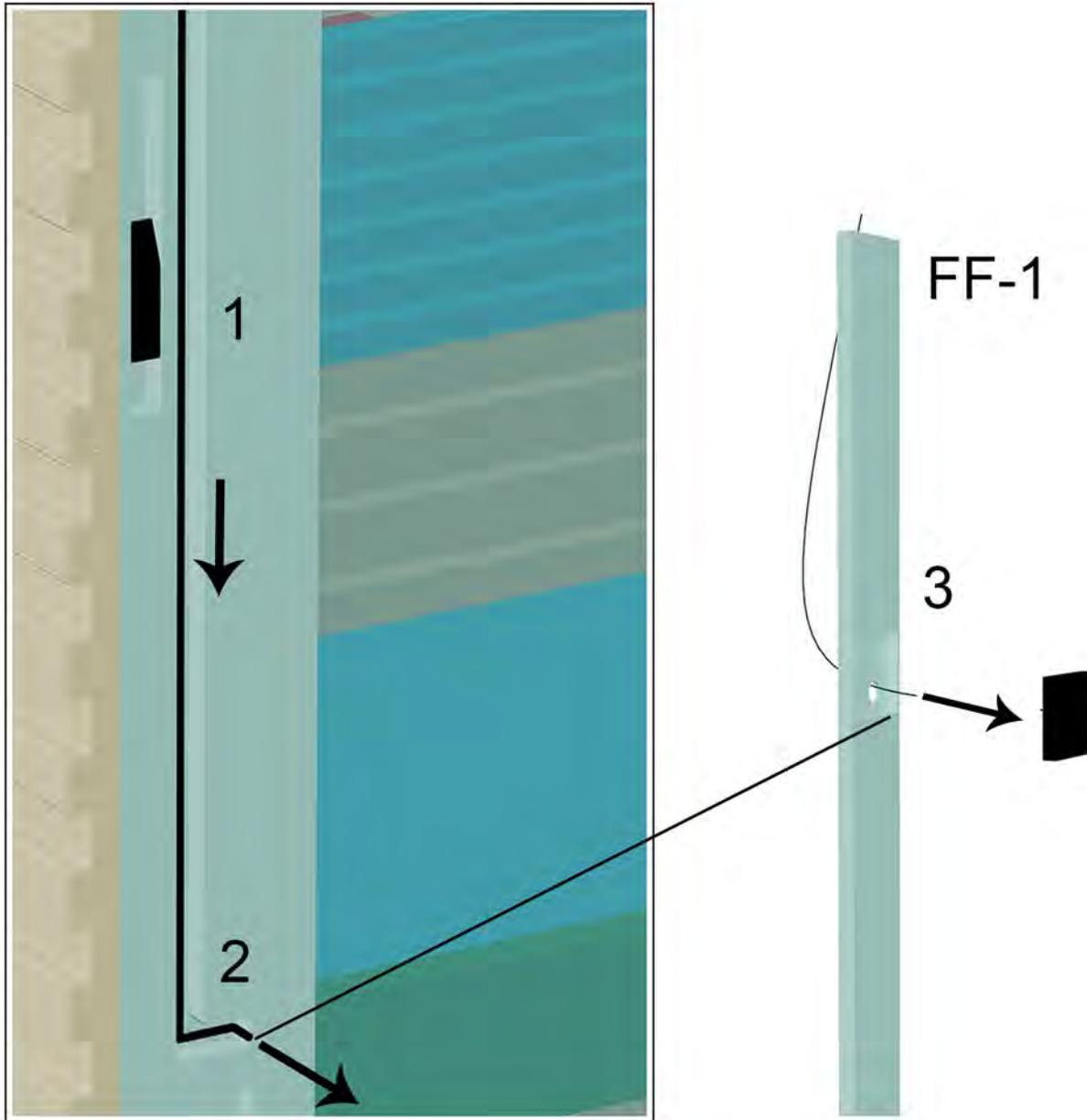
1. Put control unit cable inside (D-1) precut
